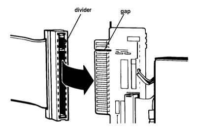
Make sure the cable connector fits properly onto the drive interface and then push it onto the interface.
